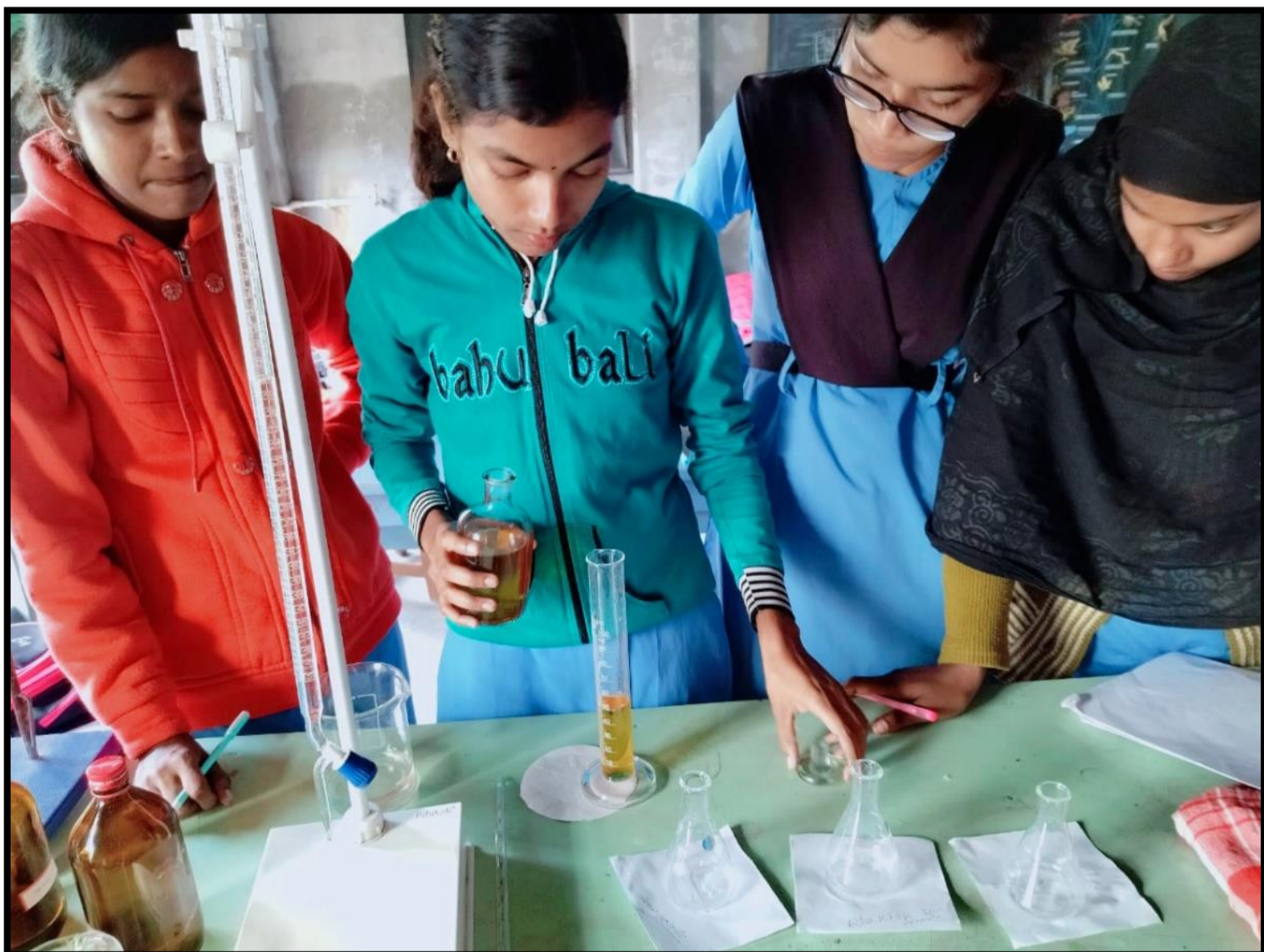
Determining the amount of dissolved oxygen in a water sample in a Zoology practical class
